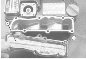
10. LVAL23373-UN: Remove Intake Cover and Gasket
