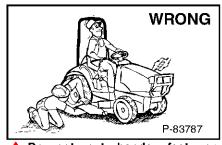
Do not put hands, feet, objects under mid-mount finish mower when engine is running.
