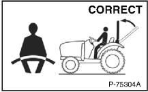
Fasten seat belt securely when Roll-Over Protective Structure (ROPS) is up and locked.
