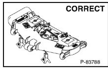
Securely block up the attachment before working underneath.
