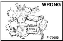
Do not use compact tractor or mid-mount finish mower atmosphere with explosive dust, explosive gas, or where exhaust can contact flammable material.
