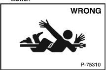
Keep all guards and shields in place. Replace if missing or damaged.
