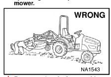
Do not put hands, feet, or objects under three-point finish mower when engine is running.
