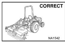
Securely block up the implement before working underneath.
