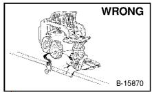
Do not undercut machine which can cause machine to fall.
