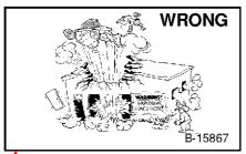
Do not use loader in atmosphere with explosive dust, gas, or where exhaust can contact flammable
