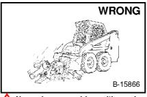
Never leave machine with engine running or with lift arms up. To park, engage parking brake and put attachment on the ground.
