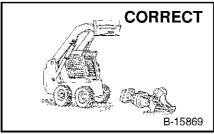
Always install approved lift arm support device when servicing loader when lift arms are raised.
