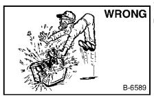
Lead-acid batteries produce flammable and explosive gases.
