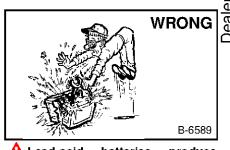
Lead-acid batteries produce flammable and explosive gases.
