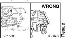
Never work on the machine with Fift arm or cargo box up unless supported by an approved support device. Replace if damaged.
