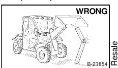
Never work on the machine with Diff arm up unless supported by an approved support device. Replace if damaged. Never work on a raised implement unless it is properly supported.
