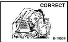
Always install approved lift arm support device when servicing the mower. Raise lift arms and tilt Bob-Tach fully forward.
