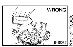
Never work on VersaHANDLER with boom up unless boom is held by an approved boom stop. Replace if damged.
