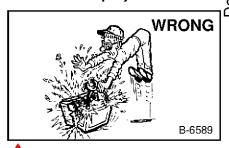
Lead-acid batteries produce flammable and explosive gases.
