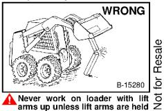
Never work on loader with lift arms up unless lift arms are held by an approved lift arm support device. Replace if damaged.
