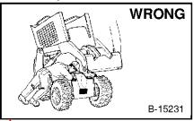
Disconnecting or loosening any hydraulic tubeline, hose, fitting, component or a part failure can cause lift arms to drop. Do not go under lift arms when raised supported bv unless approved lift arm support device. Replace it if damaged.
