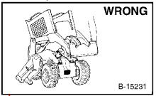
Disconnecting or loosening any hydraulic tubeline, hose, fitting, component or a part failure can cause lift arms to drop. Do not go under lift arms when raised supported by unless an approved lift arm support device. Replace it if damaged.
