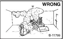
Have good ventilation when welding or grinding painted
