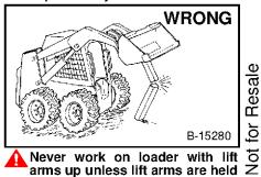
Never work on loader with lift arms up unless lift arms are held by an approved lift arm support dévice. Replace if damaged.
