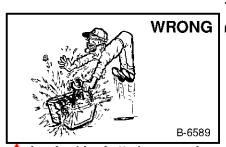
Lead-acid batteries produce flammable and explosive gases.
