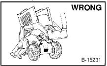
Disconnecting or loosening any hydraulic tubeline, hose, fitting, component or a part failure can cause lift arms to drop. Do not go under lift arms when raised supported bv unless approved lift arm support device. Replace it if damaged.
