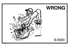
Lead-acid batteries produce flammable and explosive gases.
