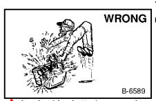
Lead-acid batteries produce flammable and explosive gases.
