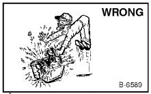
Lead-acid batteries produce flammable and explosive gases.
