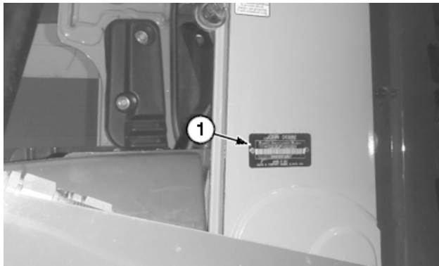
TX1140197-UN: PIN Plate Location
