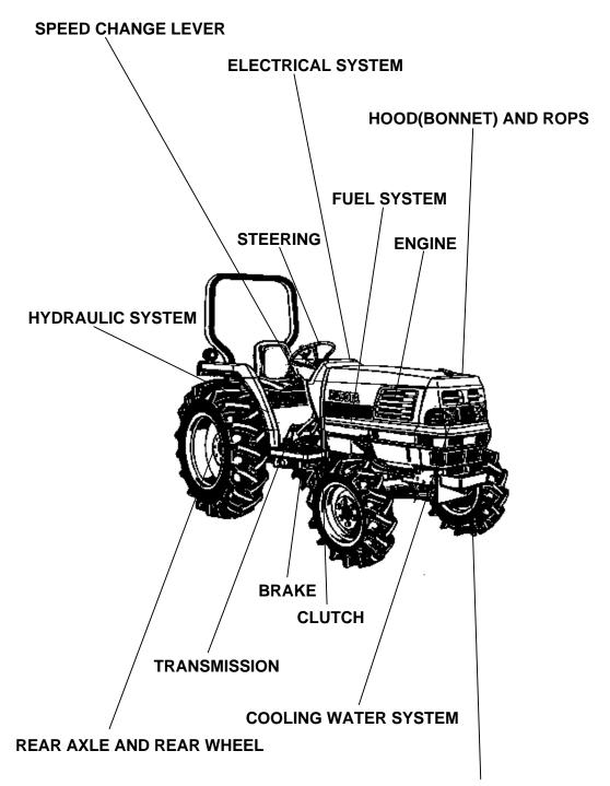
FRONT AXLE AND FRONT WHEEL AND CHASSIS
