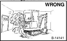
Vent exhaust to outside when engine must be run for service. Exhaust system must be tightly sealed. Exhaust Fumes can kill
