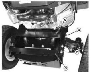
Install the top (N) and bottom (O) heat shields. Secure with two cap screws (P) and two side cap screws (Q). Tighten the four cap screws to specification (below).
