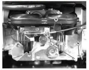
Connect retaining clamps (L). Adjust choke (M) and throttle (N) cables. See "Choke Cable Adjustment", and see "Throttle Cable Adjustment".
