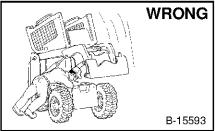
Disconnecting or loosening any hydraulic tubeline, hose, fitting, component or a part failure can cause lift arms to drop. Do not go under lift arms when raised supported unless bv approved lift arm support device. Replace it if damaged.
