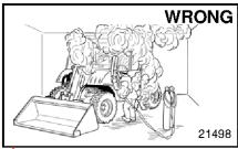
Have good ventilation when welding or grinding painted parts. Wear dust mask when grinding painted parts. Toxic dust and gas can be produced.
