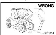
Never work on the machine with lift arm up unless supported by an approved support device. Replace if damaged. Never work on a raised implement unless it is properly supported.
