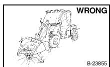
Disconnecting or loosening any hydraulic tubeline, hose, fitting, component or a part failure can cause lift arm or implement to drop. Do not go under lift arm when raised unless supported by an approved lift arm support device or under raised implement without proper supported. Replace if damaged.
