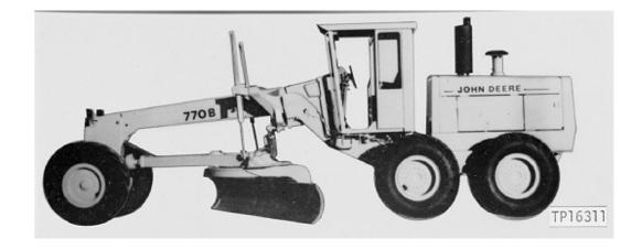
LEFT SIDE VIEW OF JOHN DEERE 770B MOTOR GRADER (MANUFACTURED 1986-1997)
