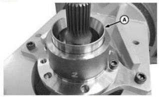
Install Outer Bearing Cup into Hub
