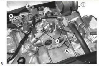
Disconnect fuel injector leads (J), water temperature lead (G), vacuum sensor lead (H), and thermo switch lead (I).
