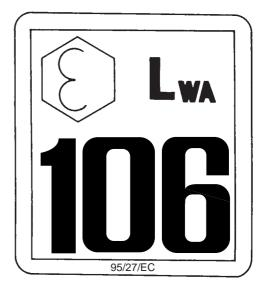
Noise level indicated is the guaranteed value as specified in the directive 86/662/EEC, as amended by 95/27/EEC
