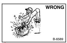
Lead-acid batteries produce flammable and explosive gases.
