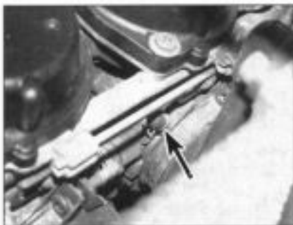
17.5b . . . and remove the blanking caps from the other unions on the carburetors
