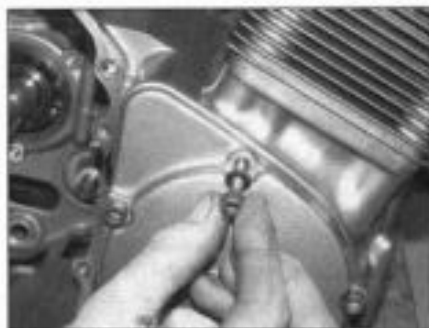
16.13b . . . and do not forget the sealing washer with the top bolt
