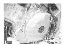
Turn the crankshaft to set the No.1 (Front) cylinder at TDC of compression stroke. (Align the "F | T" line on the generator rotor to the index mark of valve timing inspection hole and also bring the camshafts to the position as shown in page 2-8.)
