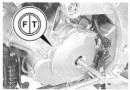
. To inspect the No.1 (Front) cylinder tappet clearance, use a thickness gauge between the tappet and the cam. If the clearance is out of specification, adjust it into the specified range.
