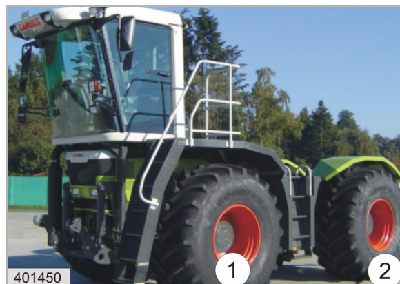
1 = Floating axle 2 = Rigid axle
