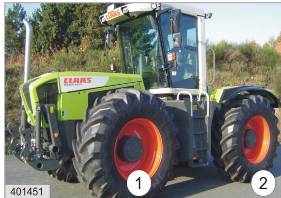
1 = Floating axle 2 = Rigid axle
