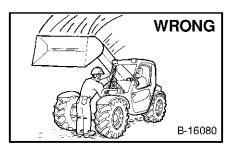
Disconnecting or loosening any hydraulic tubeline, hose, fitting, component or a part failure can cause boom to drop. Do not go under boom when raised unless supported by an approved boom stop. Replace if damaged.
