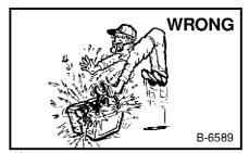
Lead-acid batteries produce flammable and explosive gases.
