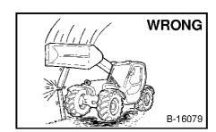
Never work on Telescopic Handler with boom up unless boom is held by an approved boom stop. Replace if damaged.
