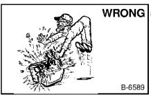
Lead-acid batteries produce flammable and explosive gases.
