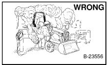
Avoid exhaust fume leaks which can kill without warning. Exhaust system must be tightly sealed.
