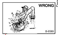
▲ Lead-acid batteries produce flammable and explosive gases.
