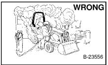
ventilation good welding or grinding painted parts. Wear dust mask when grinding painted parts. Toxic dust and gas can be produced.
