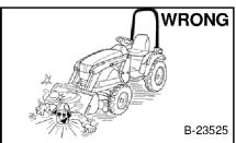
Disconnecting or loosening any hydraulic tubeline, hose, fitting, component or a part failure can cause loader arms to drop.
