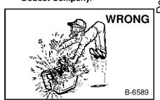
Lead-acid batteries produce flammable and explosive gases.
