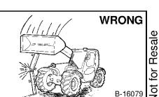
Never work on VersaHANDLER with boom up unless boom is held by an approved boom stop. Replace if damaged.
