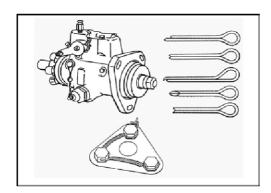
Counter pins, cotter pins and other means whenever removed must be replaced.
