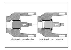
Always USE the special tool for this purpose. Where necessary, APPLY stress, by a press.
