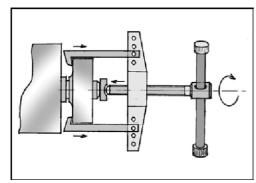
USE the appropriate pullers to pull pulleys, hubs and gears.
