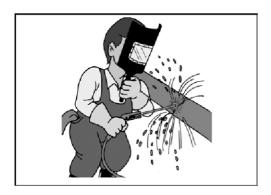
To perform welds, besides disconnecting the battery, USE the necessary protections: mask or goggles, gloves and apron. The lack of eye protection, for example, affects the eyesight in a short time, often irreversibly.
