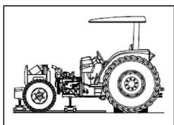
When opening the tractor, it is essential to use the appropriate trails and carts. This provides, besides safety, a profitable and quality service. Always USE wooden blocks in wedge to shim the wheels that will not be displaced for the opening.
