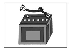
Always TURN OFF the battery negative cable, preventing someone from triggering the accidental or inadvertent starter actuation.
