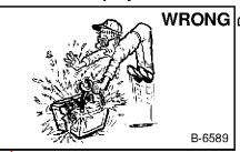
Lead-acid batteries produce flammable and explosive gases.
