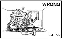
good Have ventilation when welding or grinding painted parts.
