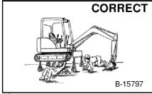
Use the correct procedure to lift and support the excavator. Always lift the blade fully before
