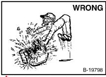
Lead-acid batteries produce flammable and explosive gases.
