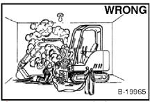
ventilation Have good when welding or grinding painted parts. Wear dust mask when grinding painted parts. Toxic dust and gas can be produced.
