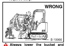
blade to the ground before doing any maintenance. Never modify equipment or add attachments not approved by
