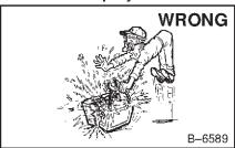
Lead-acid batteries produce flammable and explosive gases.
