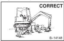
Use the correct procedure to lift and support the excavator. Always lift the blade fully before installing jackstands.
