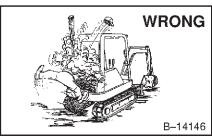
Stop, cool and clean engine of flammable materials before checking fluid.
