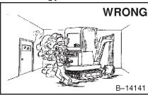
Vent exhaust to outside when engine must be run for service. Exhaust system must be tightly sealed. Exhaust fumes can kill without warning.
