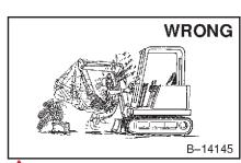
Always lower the bucket and blade to the ground before doing any maintenance.
