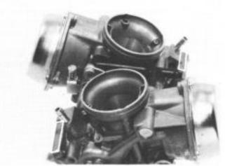
The carburetor identification number is on the carburetor body intake side.
