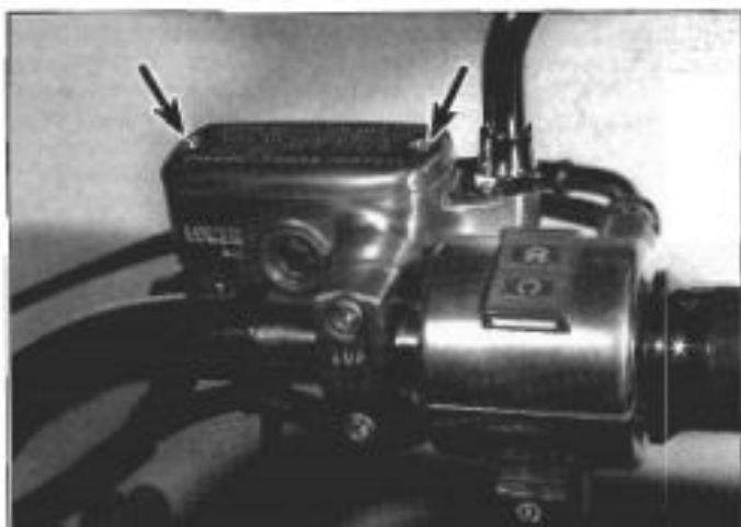
3.7a Brake fluid in the front master cylinder reservoir should be above the line next to the window; to remove the cover, remove these two screws (arrows)
