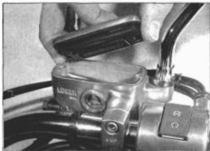
3.9 To add fluid to the front brake master cylinder, carefully remove the cover and diaphragm
