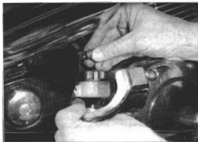
3.10 To add fluid to the rear brake master cylinder, remove the cover and unscrew the reservoir cap
