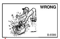
▲ Lead-acid batteries produce flammable and explosive gases.
