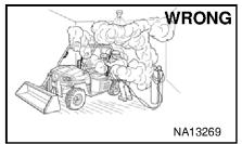
Have good ventilation when welding or grinding painted parts. Wear dust mask when grinding painted parts. Toxic dust and gas can be produced.
