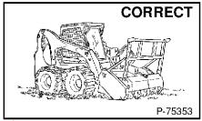
When servicing the forestry cutter always fully lower the lift arms, place the forestry cutter flat on the ground, engage the parking brake and stop the engine.
