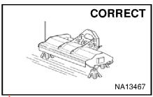
Securely block up attachment before working underneath.
