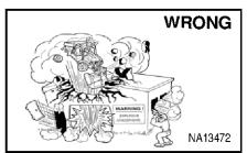
Do not use utility vehicle or mower in atmosphere with explosive dust, explosive gas, or where exhaust can contact flammable material.
