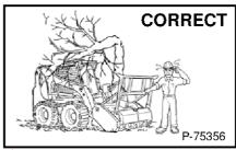
Do Not operate forestry cutter without a Level II FOPS kit installed on the cab of the loader. Do Not operate without forestry door installed.
