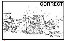
Flammable debris, can cause a fire hazard. Inspect the loader and forestry cutter and clean as necessary to avoid debris accumulation.
