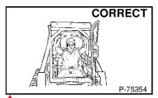
Always use the seat bar and fasten seat belt snugly. Always keep feet on the pedals when operating loader.
