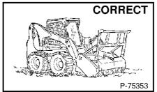
When servicing the forestry cutter always fully lower the lift When arms, place the forestry cutter flat on the ground, engage the parking brake and stop engine.
