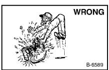
Lead-acid batteries produce flammable and explosive gases.
