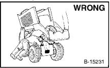
Disconnecting or loosening any hydraulic tubeline, hose, fitting, component or a part failure can cause lift arms to drop. Do not go under lift arms when raised supported unless bv an approved lift arm support device. Replace it if damaged.
