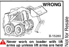
Never work on loader with lift arms up unless lift arms are held by an approved lift arm support dévice. Replace if damaged.
